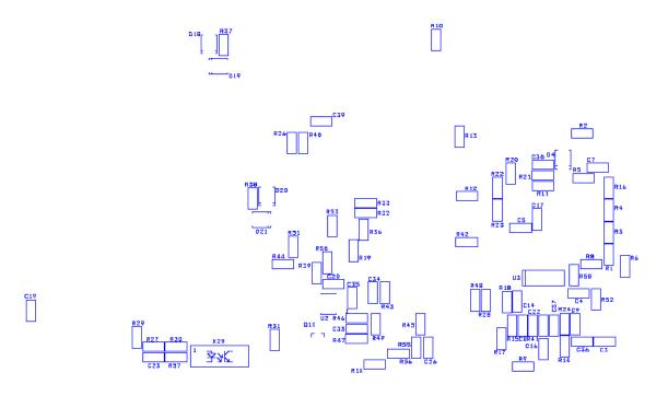
Figure 5. PCB Layout – Silkscreen Bottom
