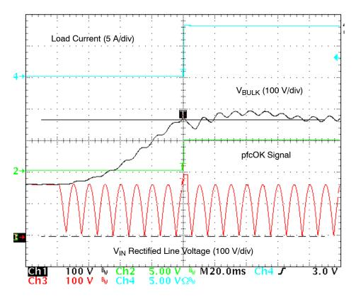
Figure 8. Startup Phase at 120 Vrms and  $I_{OUT}$  = 8 A
