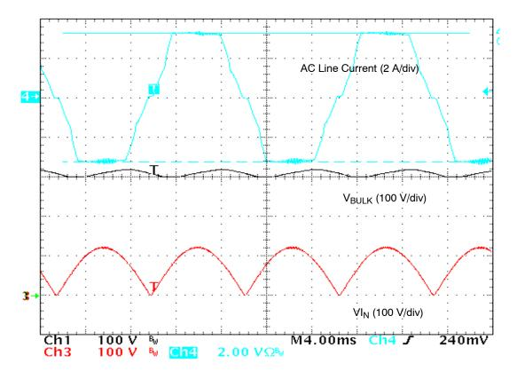
Figure 14. Action of the Overcurrent Limitation (This Test was Made by Creating an Overload Condition at 90 Vrms).
