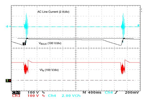
Figure 11. The Circuit Enters a Safe Low Duty–Cycle Hiccup Mode if the 19 V Output is Short Circuited (Test Made at 120 V<sub>RMS</sub>)
