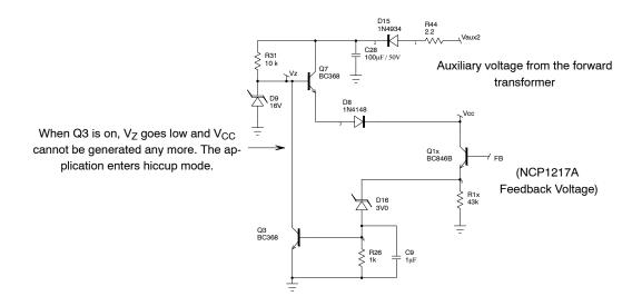
Figure 13. Circuit for Overload Protection
