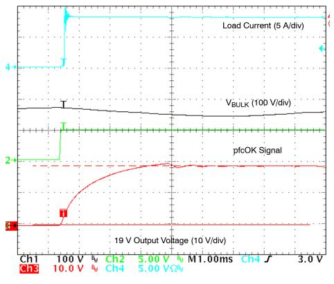
Figure 10. Startup Phase at 120 Vrms
