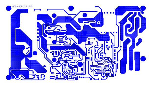
Figure 6. PCB Layout – Bottom Layer
